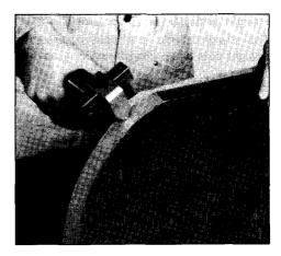
Install the trimmer guide on the guide holder with the wing bolt. Then use the hex wrench to loosen the bolts on the tool base and insert the guide holder into the grooves in the tool base. Adjust the distance between the bit and the trimmer guide and tighten the bolts securely.
